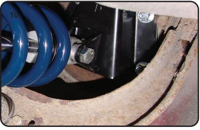
Tighten the lower Coilspring Adjusting nut until the Coilspring is sitting snuggly on the CoilOver. Using the Spanner wrench add another 1/2" of preload in the spring by threading the adjuster nut up the Shock Body. Be sure that the locking screw is lightly tightened in the adjuster nut. Once you have preloaded tighten the locking screw. It may be necessary to add more preload, this will be determined once the car is setting on the ground.
