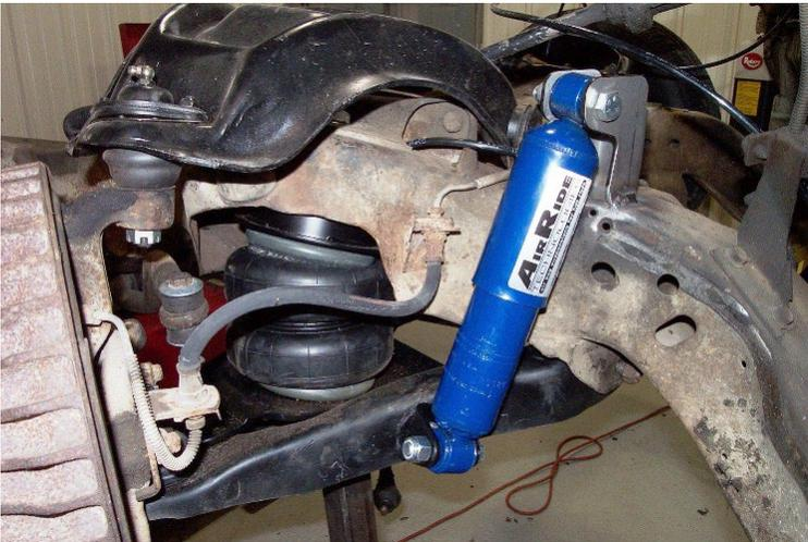
1. The upper shock mount must be welded to the frame. It may need to be cut down to match the stroke of the air spring and suspension. Make sure that when the suspension is fully compressed that the shock is about  $\frac{1}{4}$ " from being fully compressed.
