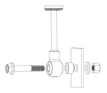
2. Attach the shock to the axle using the new shock bolt kit supplied.
