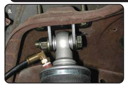
**8.** Fasten the ShockWave to the upper bracket using a  $\frac{1}{2}$ " x 2  $\frac{1}{2}$ " bolt and Nylok nut.  $\frac{1}{2}$ " I.D. aluminum spacers must be installed on each side of the bearing. Torque to 75 ftlbs.
