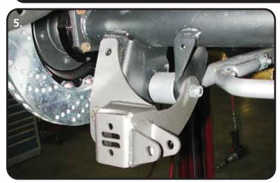
**5.** Remove the lower trailing arm mounting bolt. (Do one side at a time to keep the axle from rotating). Install the longer  $\frac{1}{2}$ " x 3  $\frac{3}{4}$ " bolt through the lower trailing arm from the outside in. Install the lower bracket over the bolt and secure with a  $\frac{1}{2}$ " Nylok nut and flat washer. Snug the Hardware, but do NOT fully tighten at this time.
