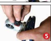
Once the knob is removed slide a Delrin washer over the eyelet. Next, slide the upper spring mount (803-00-199) over eyelet as seen in figure 4.
