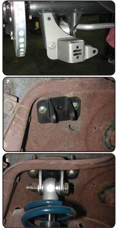
**6.** The lower bolt hole in the back of the bracket will align with the factory shock stud hole. Use a  $\frac{1}{2}$ " x 1  $\frac{1}{2}$ " bolt, Nylok nut and flat washers. The upper hole must be drilled with a  $\frac{1}{2}$ " bit. The edge of the bracket should be parallel to the axle bracket. Use an centering punch and 1/8" bit to drill a pilot hole. A  $\frac{1}{2}$ " x 1  $\frac{1}{2}$ " bolt, Nylok nut and flat washers will be used here as well. Torque all hardware to 75 ftlbs.
