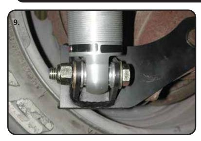
**9.** Fasten the CoilOver to the lower bracket using a  $\frac{1}{2}$ " x 2  $\frac{1}{2}$ " bolt, 1/2" flat washer, and Nylok nut.  $\frac{1}{2}$ " I.D. aluminum spacers must be installed on each side of the bearing. Torque to 75 ftlbs.
