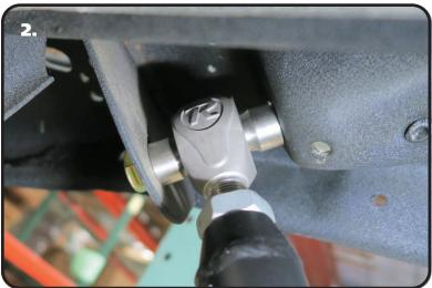
2. Insert the R-Joint end of the upper StrongArm into the OEM location, making sure the StrongArm is positioned correctly. Use the illustration on **Page 2** to help determine the correct orientation. Line up the through hole of the R-joint with the upper control arm mounting holes. Insert a 1/2"-13 x 3 1/2" hex bolt through the holes. Install a 1/2" flat washer and 1/2"-13 nylok nut on the threads of the bolt sticking through the frame. Torque to 75 ftlbs.
