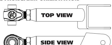
THIS ILLUSTRATION SHOWS HOW THE UPPER STRONGARM IS TO BE INSTALLED IN YOUR A-BODY. BOTH UPPER STRONGARMS ARE OFFSET TO <u>SAME</u> SIDE. THIS DESIGN IS BASED OFF THE OEM CONTROL ARMS TO KEEP THE DIFFERENTIAL CENTERED.
