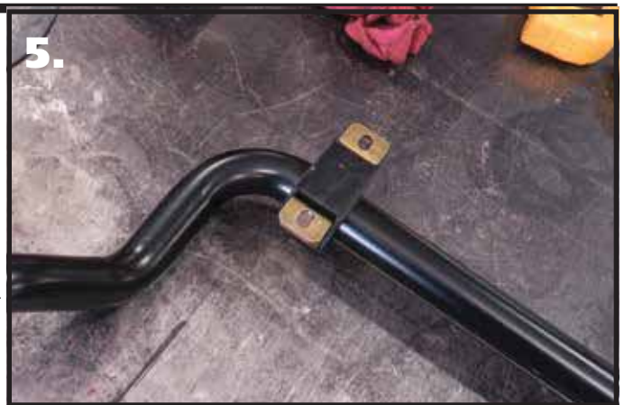
6. Slip the Bushing Straps over the Sway Bar Bushings.
