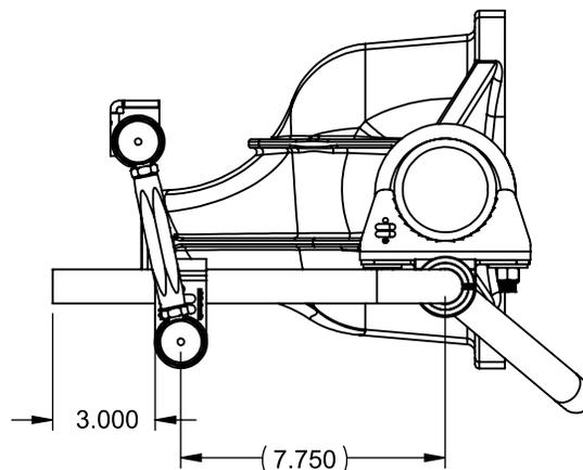
**13.** We recommend getting the swaybar as level as possible at ride height and with no preload. Both of these steps are done by adjusting the end links. These end links can be adjusted from 6" to 6 3/4". Disconnect the end links from the swaybar and adjust one side to get the swaybar level. Reattach the end link to the swaybar and adjust the 2nd end link so that it goes in and out of the clamp-on mount with ease. This will be zero preload.
