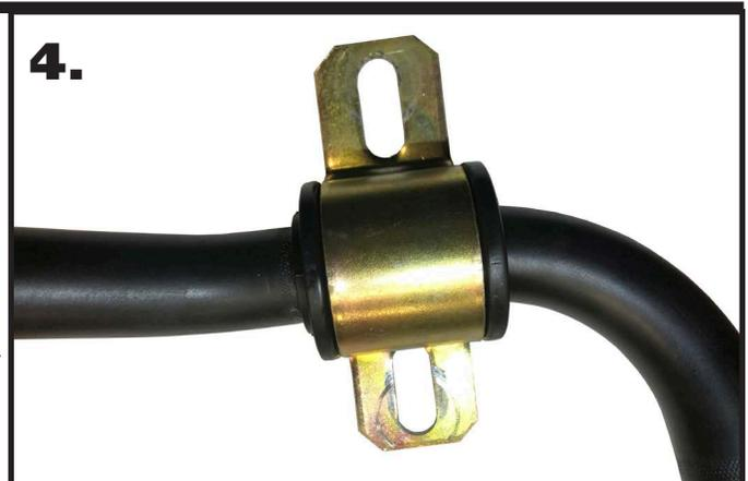
**4.** Install the bushing straps over the sway bar bushings.
