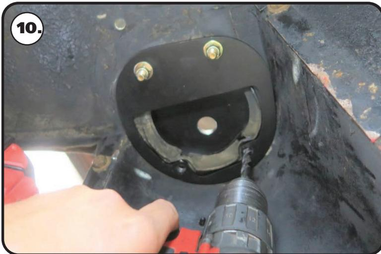
**10.** Drill the inner (2) holes using a 5/16" drill bit. Install a 5/16" on each of (2) 5/16"-18 x 1 3/4" hex bolts. Insert the bolts/ washer through the inner 2 holes. Install a 5/16" flat washer & 5/16"-18 nylok nut on each bolt. Torque the hardware to 25 ft-lbs.
