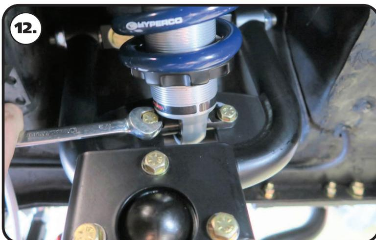
**12.** Raise the upper arm up to the CoilOver. Line up the shock mounting holes with the through hole of trunnion. Install a 5/16" flat washer on each of (2) 5/16"-18 x 1 1/4" hex bolts. Insert the bolt/washers in the aligned holes. Install a 5/16" flat washer and 5/16"-18 nylok nut on the threads of each bolt. Torque to 25 ft-lbs.
