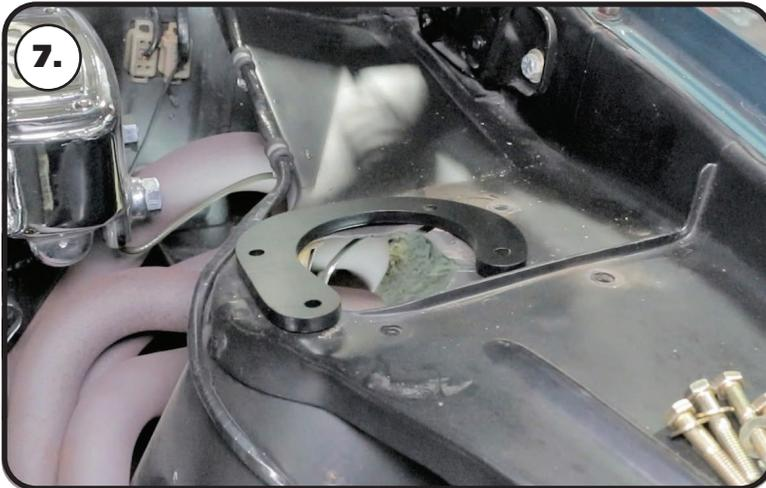
7. The kit includes an upper spacer due to different metal thicknesses at the upper shock mounting area. Place the upper spacer on top of the shock tower with the opening to the FRONT of the car and the curves side toward the engine. The mounting holes will align with the outer slots of the upper shock mount.
