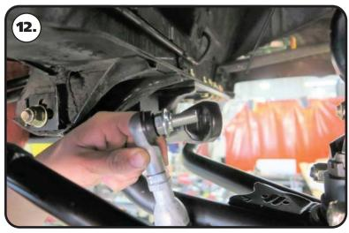
**12.** Install a t-bushing on the lower 90 degree end link. The t-bushings are installed with the large diameter against the shoulder of the end link. Insert the 90 degree end link/t-bushing into the swaybar end with the threads pointing toward the spindle.
