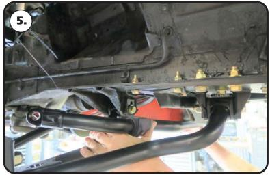
**5.** Insert the sway bar into position. The front bolt of the sway bar bushing/spacer will align with the rear inner bolt of the crossmember.
