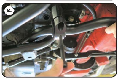
**8.** With the sway bar lined up with the front mounting hole. Install a 3/8" x 5/8" OD flat washer on (2) 3/8"-16 x 3 1/2" socket head cap screw. Insert the bolt/washer in the front hole of the bushing strap and spacer.
