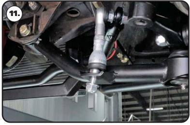
**11.** Insert the straight end of the PosiLink into the sway bar tab of the lower control arm. Install a 12mm flat washer and M12-1.75 nylok nut on the threads of the PosiLink.
