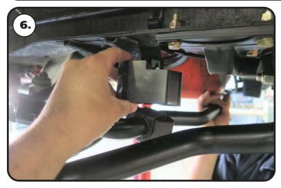
**6.** The supplied spacer needs to be installed between the bushing/strap and frame. The spacer is stepped on the frame side. The notch will be to the front of the car.
