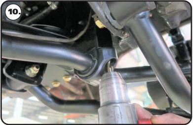
**10.** Use the bushing mount as a guide to drill a 3/8" hole in the frame for the rear hole.
