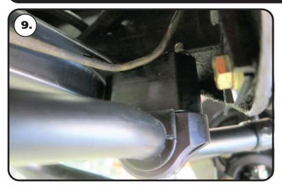
**9.** Install a 3/8" SAE flat washer & 3/8"-16 nylok nut on the threads of the bolt. Snug the hardware down to hold the sway bar in place.
