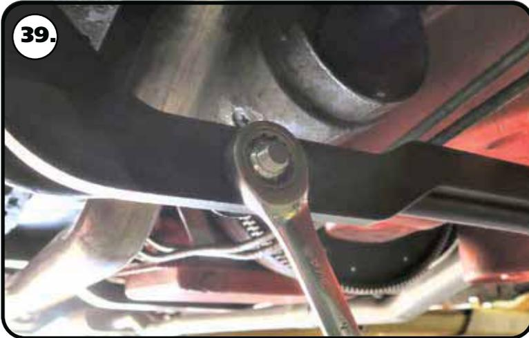
**39.** Install the draglink adapter on the studs sticking out of the OEM draglink. Install a 1/2"-20 mechanical locking nut on the threads of each stud sticking through the draglink adapter. Torque the nuts to 50 ft-lbs.
