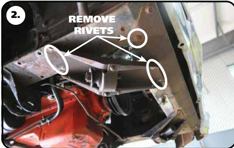
2. The OEM strut rod mounts will need to be removed from the car. The strut rod mount is attached to the car with 4 rivets. There is a 5th rivet that attaches the radiator support to the frame rail that will also need removed. We have seen some cars that have a bolt/nut here instead of a rivet.
