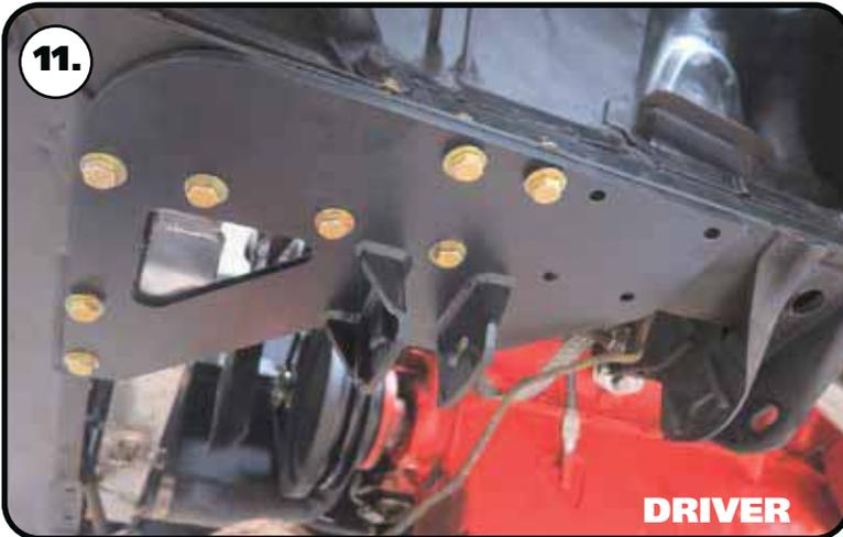
**11.** Install a 7/16" flat washer on each of (4) 7/16"-14 x 1 1/4" bolts. Insert the bolts/washers in the holes that align with the holes that were just drilled. The threads of the bolts need to be pointing up. Install a 7/16" flat washer and 7/16"-14 nylok nut on each of the bolts. Torque the bolts to 80 ft-lbs. Repeat Step 8-12 on the other side.
