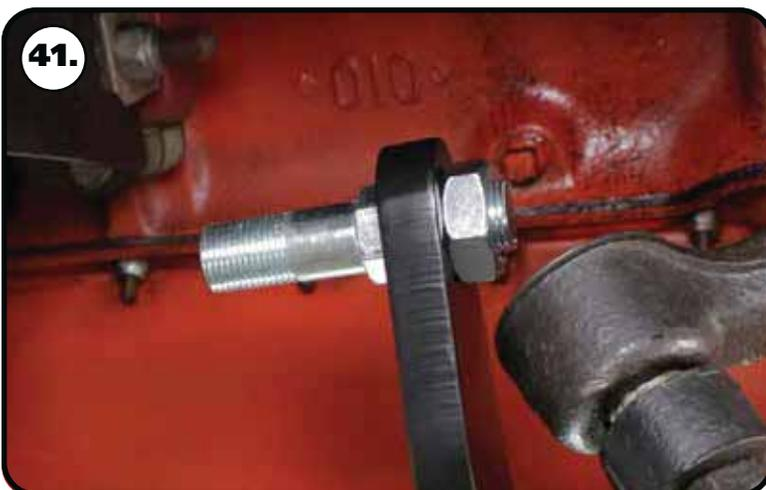
**41.** Install the 5/8"-18 **THIN** mechanical locking nut on the threads of the stud sticking through the centerlink adapter and torque to 45 ft-lbs.
