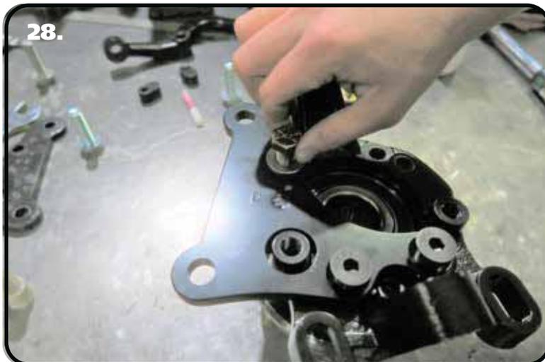
28. Insert a 1/2"-13 x 1 1/4" flat head socket cap screw in each of the lower mounting holes. Install a 1/2" flat washer on a 1/2"-13 x 1 1/4" hex bolt and insert it in the upper mounting hole. Tighten the hardware to 75 ft-lbs.
