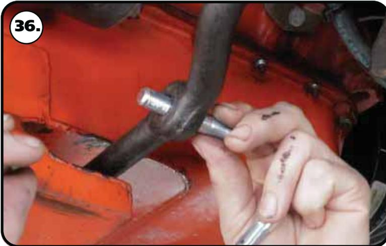
**36.** The SMALL tapered studs will get installed into the factory centerlink with the taper going into the centerlink, a 7/16" castle nut is used to attach it to the centerlink. The straight shank will point to the front of the car.
