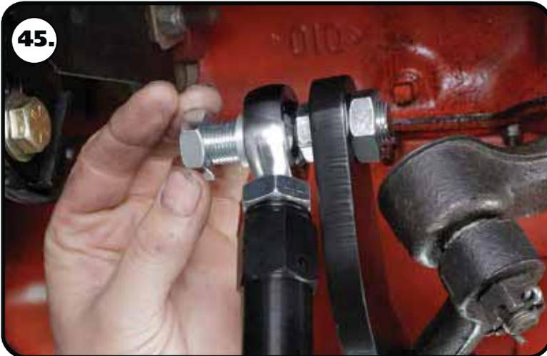
**45.** Install the 5/8" ID x .125" spacer on the stud followed by a 5/8"-18 mechanical locking nut. Torque to 45 ft-lbs.
