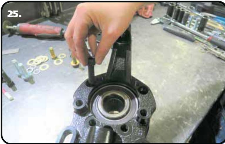
**25.** The Hub is attached to the spindle using (3) M12-1.75 x 40 SHCS. Apply RED Loctite to each of the mounting bolts. Insert them into the correct holes and Torque to 99 ftlbs.
