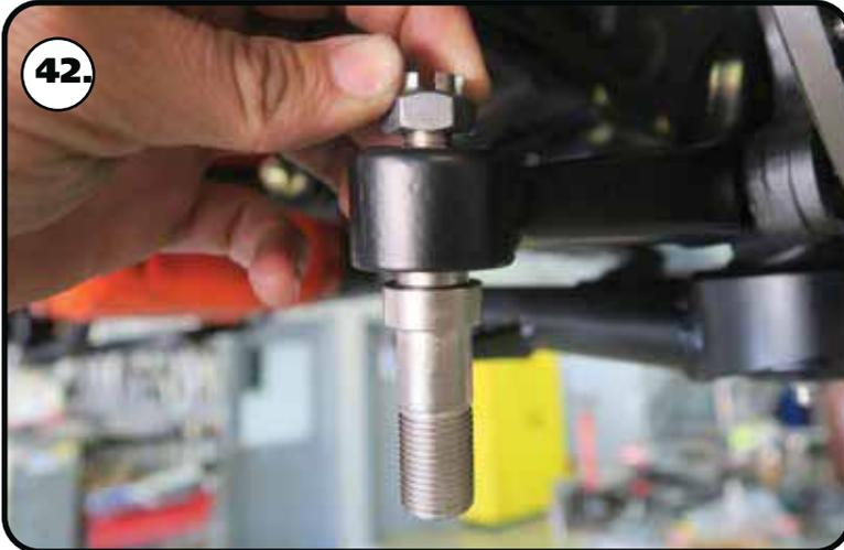
**42.** Install the stud with the round flange into the steering arm with the taper going into the steering arm. Torque the nuts to 35 ft-lbs and tighten as needed to align cotter pin hole and install cotter pin.
