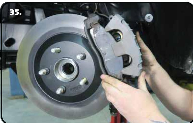
**35.** Install the brake pads and caliper.
