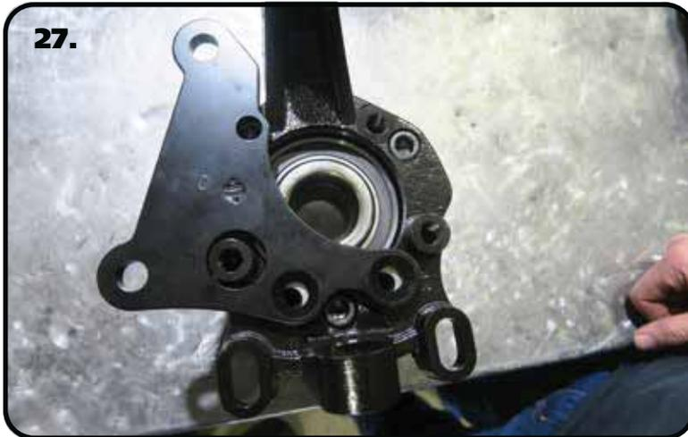
27. The caliper brackets are side specific. They have a D & P stamped in them. Lay the correct side caliper bracket on top of the shims, aligning the mounting holes with the mounting holes of the bracket. The counter sunk holes should facing up.
