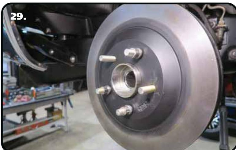
29. Install the rotor on the hub. Thread some lug nuts on the threads of the hub to hold the rotor tight on the hub.
