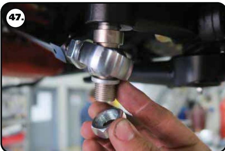
**47.** Install the 5/8" ID x .125" spacer on the stud followed by a 5/8"-18 mechanical locking nut. Torque to 45 ft-lbs.
