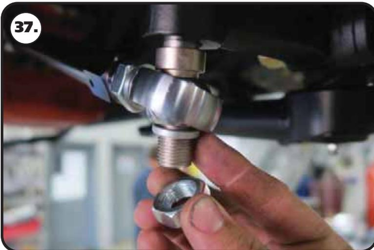
**37.** Install the 5/8" ID x .125" spacer on the stud followed by a 5/8"-18 mechanical locking nut. Torque to 45 ft-lbs.
