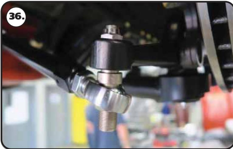
**36.** Install a 5/8" ID x 3/8" spacer on the steering arm stud, followed by the outer end of the tie rod.
