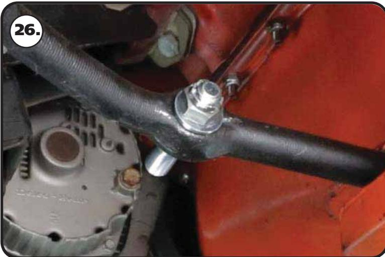
**26.** Torque the nuts to 35 ft-lbs and tighten as needed to align cotter pin. Install cotter pin and bend the ends.
