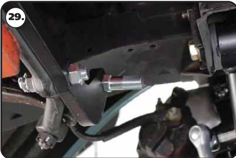
**29.** The studs with the short hex get installed into the centerlink adapter. The short side goes into the adapter attached with the 5/8"-18 thin top lock nut, with the long side of the stud pointing forward.
