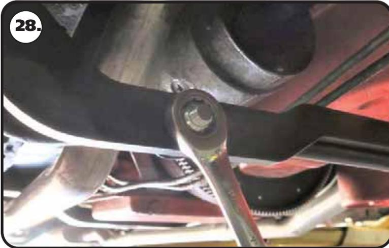
**28.** Install the draglink adapter on the studs sticking out of the OEM draglink. Install a 1/2"-20 mechanical locking nut on the threads of each stud sticking through the draglink adapter. Torque the nuts to 50 ft-lbs.
