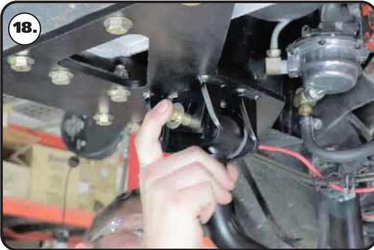
**18.** Install a 1/2" flat washer on each of (4) 1/2"-20 x 4" hex bolt. Insert the bolt in the eccentric eliminator plate. Install the assembly in the lower control arm mount. Repeat for the 2nd bushing.
