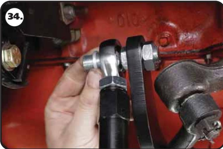
34. Install one end of the tie rod onto the stud of the centerlink adapter.
