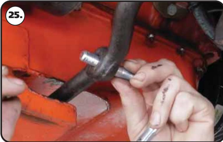
**25.** The SMALL tapered studs will get installed into the factory centerlink with the taper going into the centerlink, a 7/16" castle nut is used to attach it to the centerlink. The straight shank will point to the front of the car.
