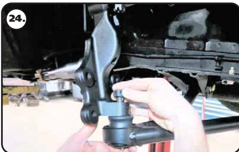
**24.** The spindles included in this kit are identical for each side. They are not side specific until the steering arm is attached. Install the spindle on the lower ball joint pin. Torque the ball joint castle nut to 65 ft-lbs and tighten to align the cotter pin holes. Install the cotter pin in the ball joint pin hole and bend the ends of the cotter pin to hold it in place. Install the grease zerk supplied with the ball joint.
