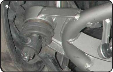
**9.** Attach the spindle to the control arms.
