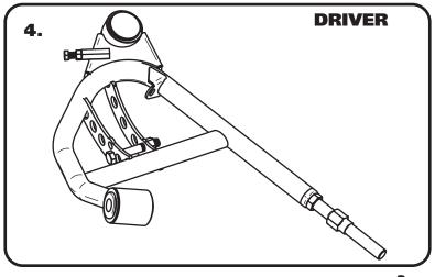
**4.** The control arms are marked "D" for Driver and "P" for Passenger. The ball joint pin points down and the sway bar mount is on the front side of the arm.
