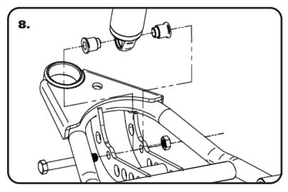
**8.** Insert the bearing spacers into the lower shock bearing. The SMALL end goes into the bearing. Swing the control arm up, line up the 1/2" holes with the bearing spacers, insert 1/2"-13 x 3 1/2" bolt. Install a 1/2" flat washer and nylok nut. Torque to 75 ft-lbs.
