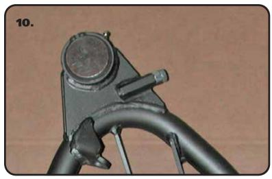
**10.** Thread the 3/8"-16 nut onto the 3/8"-16 x 1 ¼" bolt. Thread it into the front hole of the ball joint plate. You will need to adjust the steering stop to suite your needs. This setting will vary depending on wheel and tire size and other suspension components. Torque to 16 ft-lbs.
