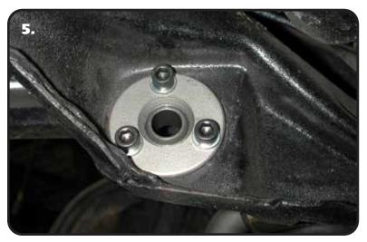
**5.** Using the bearing retainer as a template; drill three 3/8" holes in the frame to secure the assembly. Use three 3/8" x 1  $\frac{1}{4}$ " SHCS and lock washers to secure the assembly. Torque to 30 ft-lbs.
