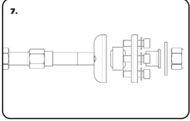
**7.** The front leg of the lower arm will attach to the frame in place of the strut rod. Refer to **Diagram 7** for assembly order. Torque the 3/4"-16 nut to 75 ft-lbs.
