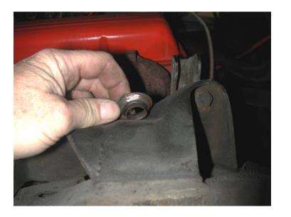
4. Surrounding the hole that the factory shock stem went through is a bushing cup. This must be removed using a chisel or air hammer.
