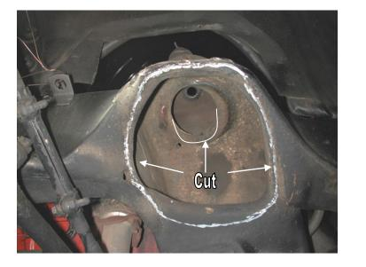
2. The inside lip of the pocket must also be remove to allow for Shockwave bellow clearance.
