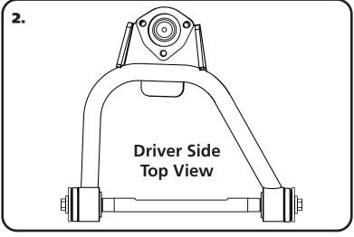
**3.** The upper control arm is attached to the factory frame using factory hardware. The driver side arm is shown in **Figure "3"**. The Ball joint is located on the arm to the REAR of the car.
