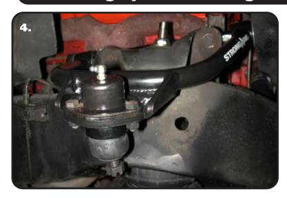
**4.** The upper control arm is attaching the factory mount using factory hardware. Reinstall the shims in the location they were removed from. The passenger side arm is shown in **Figure "4"**. Torque the mounting hardware 65-80 ft-lbs.
