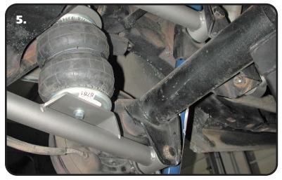
**3.** Clean the bushing surfaces on the frame and axle brackets. Lubricate with the lithium grease supplied. Fasten the front of the lower StrongArms to the frame using the 5/8" x 4" bolts, flat washers, and nylok nuts supplied. Tighten the bolts/nuts enough to eliminate any gaps.
