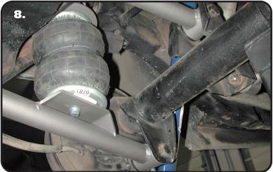
**8.** Thread the 3/8"-16 x 3/4" bolt with washer and lock washer about half way into the air spring. Slide bolt into slot on lower arm and tighten.
