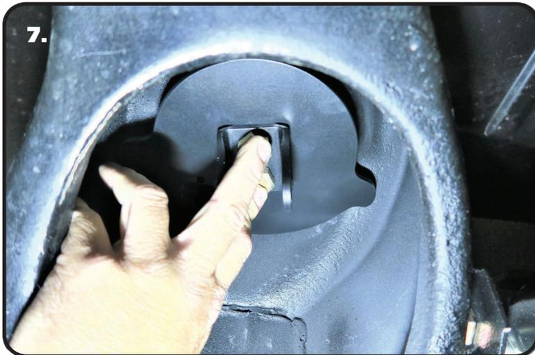
7. Position the Shock Mount/Plate up into the frame, holding the shock mount and hardware in place. **Position the mount with the tabs to the front of the car and Ridetech Icon toward the wheel.** You will need to align the upper clamp plate with the bolts that are sticking up through the frame.
