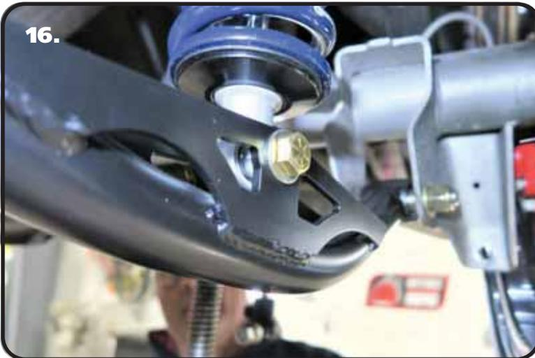
**16.** Insert the shock into the lower control arm with the adjuster knob to the front of the car. Line up the holes of the mount and shock. Install a 1/2" flat washer on a 1/2"-13 x 2 3/4" bolt. Insert the bolt/washer into the upper mount/shock. Install a 1/2" flat washer and 1/2"-13 nylok nut and Torque to 50 ftlbs.
