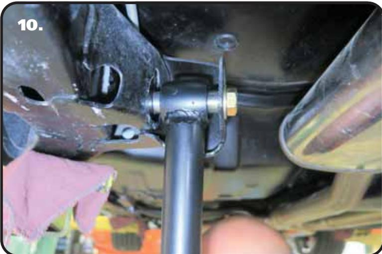
**10.** Install a 5/8" Flat Washer on a 5/8"-18 x 4" bolt. Insert the bolt/washer into the frame/R-Joint of the lower bar. Install a 5/8" flat washer and 5/8"-15 nylok nut on the threads of the bolt sticking through the frame. Tighten the hardware to eliminate any gaps.
