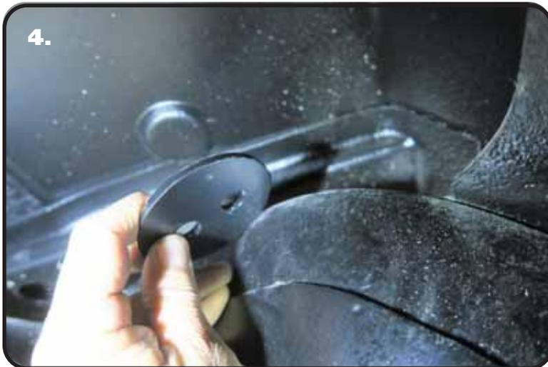
4. The Upper Clamp Plate needs to be placed on the top side of the OEM coilspring pocket. It will fit down in the recessed area of the coilspring pocket. Use **Images 4 & 5** as a reference to install the upper clamp plate.
