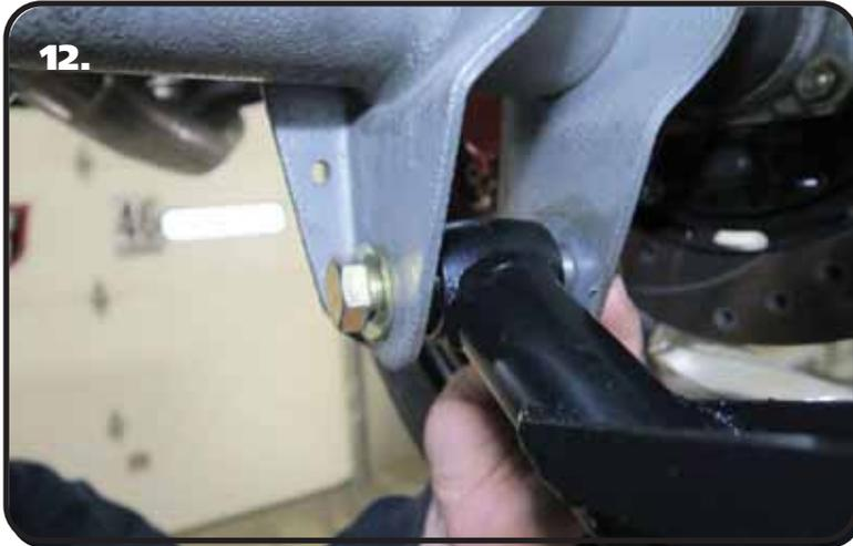
**12.** Install a 5/8" flat washer on a 5/8"-18 x 4" bolt. Insert the bolt/washer through the mounting hole. Install a 5/8" flat washer and 5/8"-15 nylok nut on the threads of the bolt sticking through the axle mount. Tighten the hardware to eliminate any gaps
