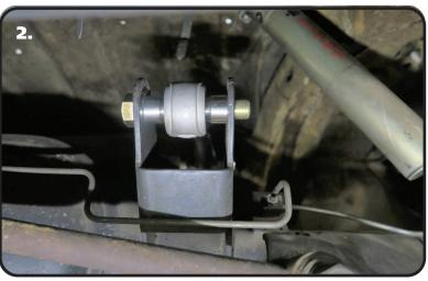
2. Install a 5/8" flat washer on a 5/8"-18 x 4" hex bolt through the mount and control arm R-Joint. Install a 5/8" flat washer, followed by a 5/8"-18 nylok jam nut onto the threads of the bolt. Tighten the hardware enough to eliminate any gaps.
