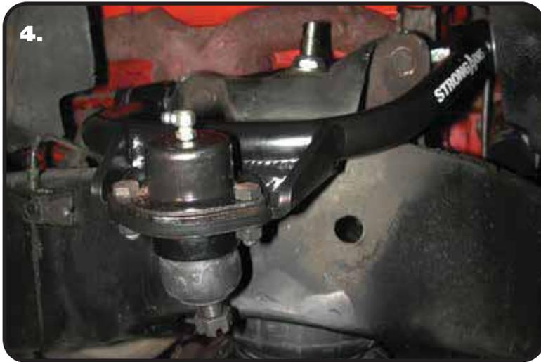
4. The Upper Control Arm is attaching the factory mount using factory hardware. Reinstall the shims in the location they were removed from. The passenger side arm is shown in **Figure "4"**.
