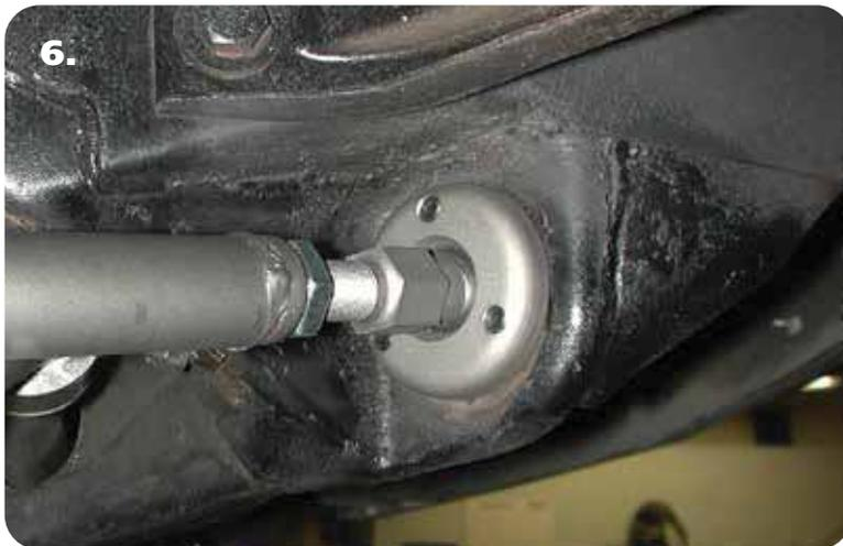
6. Insert the front leg of the control arm into the frame swivel bearing. Bolt the lower StrongArm to the frame using the factory bolt. **The lower control arm pivot bolt gets torqued to 100-125 ft-lbs when the car is sitting on the ground.**
