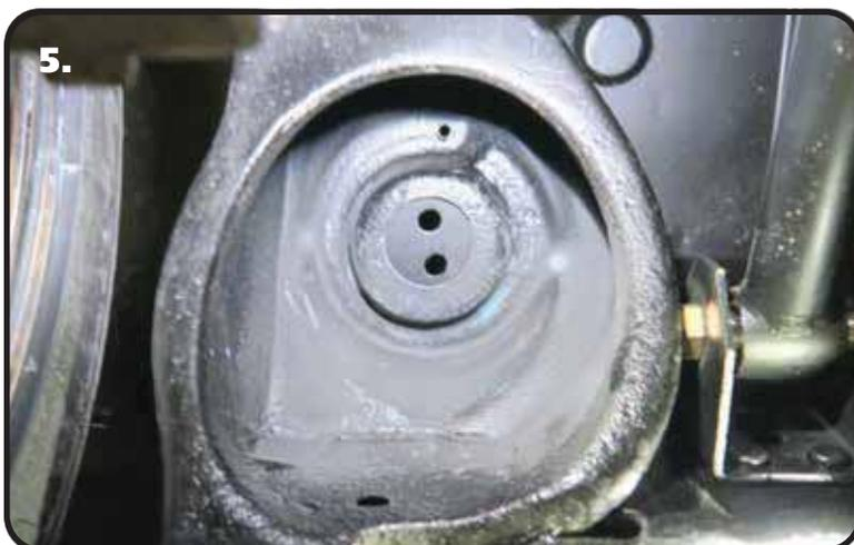
5. **Image 5** shows the Upper Clamp Plate in poistion as looking at it from the bottom side of the frame. Don't worry about the orientation of the bolt holes. You will position it correctly during the intallation of the Upper Shock Mount.
