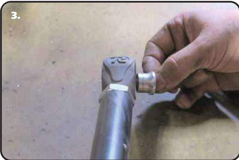
**3.** Install the 3/4" jam nut onto the end of the R-Joint end, then screw R-Joint end into the end of the panhard bar. Set the Panhard Bar to 35.750". You may need to readjust it after getting the car set at ride height, but this is a good starting point. Press the SMALL diameter of the 9/16" I.D. R-Joint spacers into each side of the center ball of the remaining R-Joint. Push the spacers in until they bottom out in the center ball.
