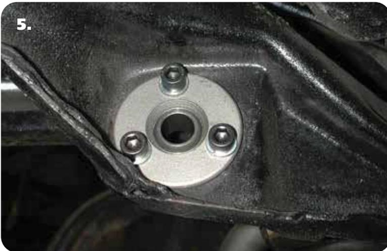
5. Using the bearing retainer as a template; drill three 3/8" holes in the frame to secure the assembly. Use three 3/8" x 1 1/4" SHCS and lock washers to secure the assembly. Torque to 30 ft-lbs.
