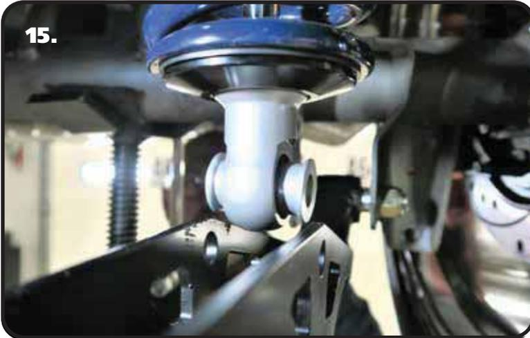
**15.** Insert the LONG shock bearing t-bushings into the bearing of the shock eyelet. The SMALL diameter of the t-bushings will insert into the shock bearing.
