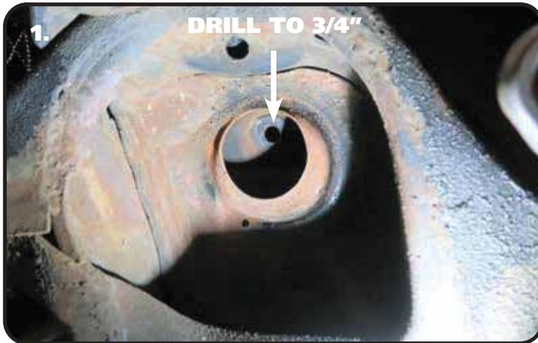
1. Drill the OEM shock hole out to 3/4". This can be done with a Unibit.
