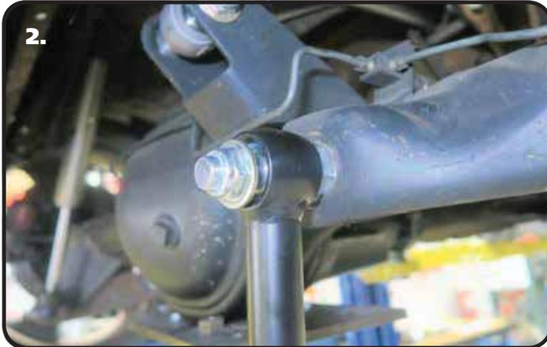
**2.** Install a Narrow 5/8" ID R-joint Spacers into each side of the R-joint of either end of the Panhard Bar. The Small Diameter goes into the R-joint. Slide the R-joint onto the stud and fasten in place with a 5/8" flat washer and 5/8"-18 thin jam nylok nut. Torque to 95 ftlbs.
