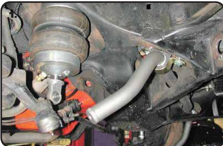
1. Slide the sway bar through the same holes in the frame that the factory bar went through. The sway bar needs to be installed with the center dropping down toward the ground to clear the engine.
