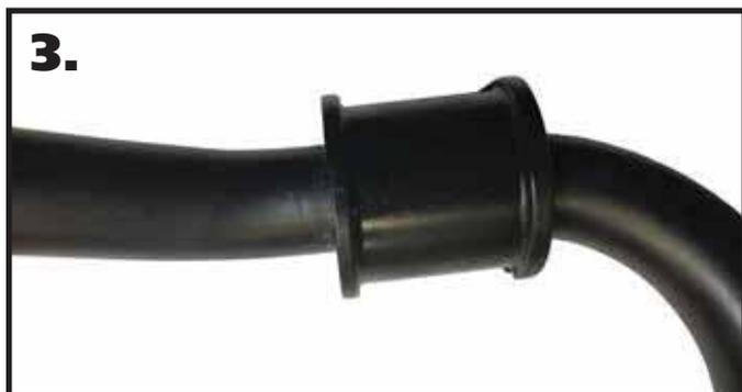
**3.** Open the sway bar bushing at the split and slip it **OVER** the sway bar. Do this for both bushings.
