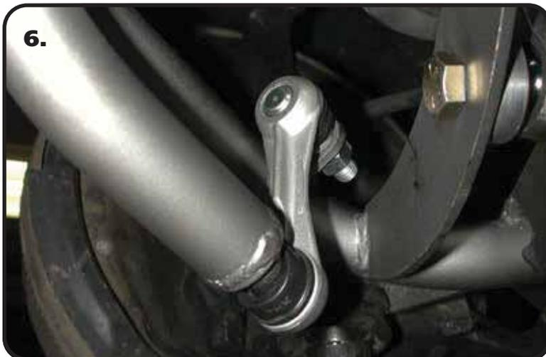
6. The other end of the PosiLink will attach to the tab on the StrongArm using a flat washer on each side of the tab and M12-1.75 nylok nut.
