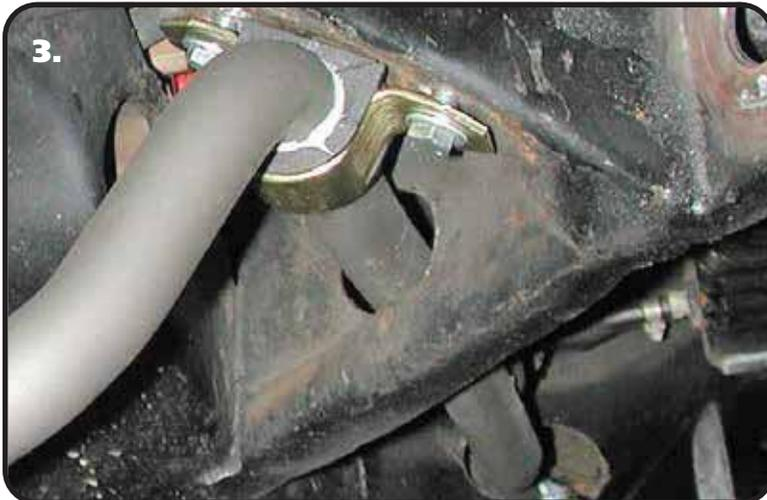
3. Clamp the sway bar up to the frame using a couple "C" clamps. The sway bar should be centered in the hole through the frame.
