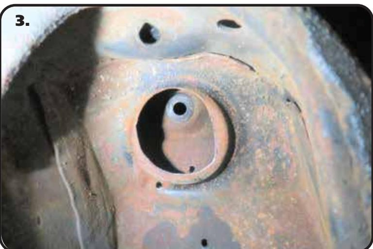
3. **Image 3** shows the spring retainer trimmed out.
