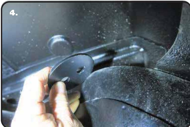
4. The The Upper Clamp Plate needs to be placed on the top side of the OEM coilspring pocket. It will fit down in the recessed area of the coilspring pocket. Use **Images 4 & 5** as a reference to install the upper clamp plate.
