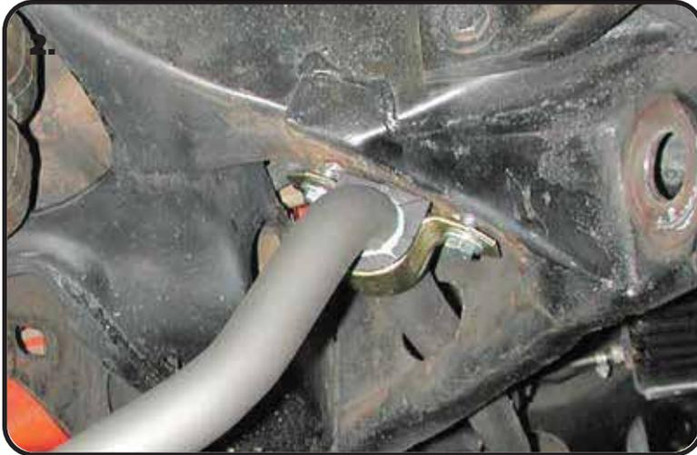
2. Lubricate the sway bar busing with the lithium grease supplied. Install the new polyurethane bushing and strap over the sway bar.
