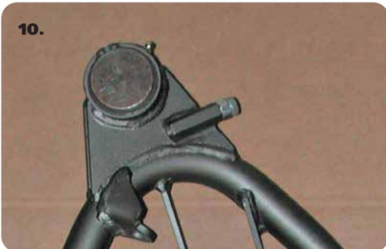
10. Thread the 3/8"-16 nut onto the 3/8"-16 x 1 1/4" bolt. Thread it into the front hole of the ball joint plate. You will need to adjust the steering stop to suite your needs. This setting will vary depending on wheel and tire size and other suspension components. Torque to 16 ft-lbs.
