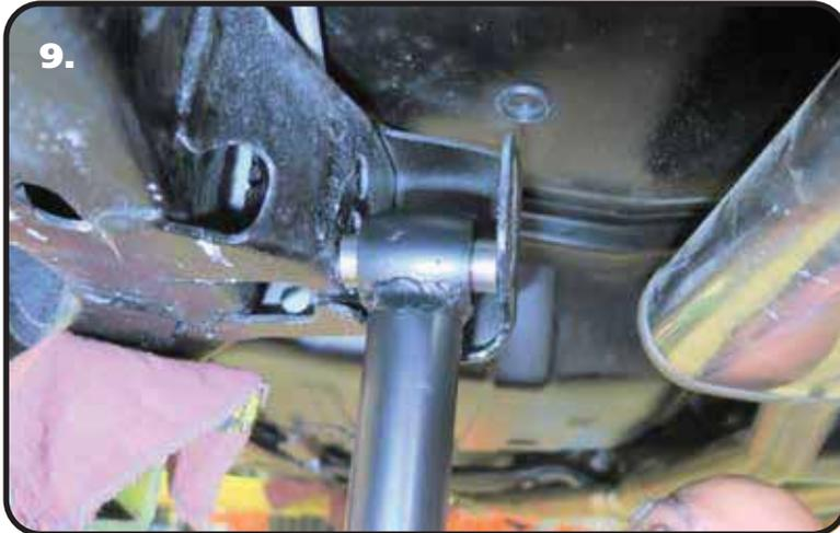
9. The Lower Control Arm has the bottom CoilOver mount built in. It will need to be installed with the CoilOver mount up and to the rear of the car. Install a 5/8" ID R-joint Spacer into the front R-joint. The Small Diameter goes into the R-joint. Slide the R-joint into the OEM lower control arm mount. Align the holes in the frame with the thru-hole of the R-Joint.
