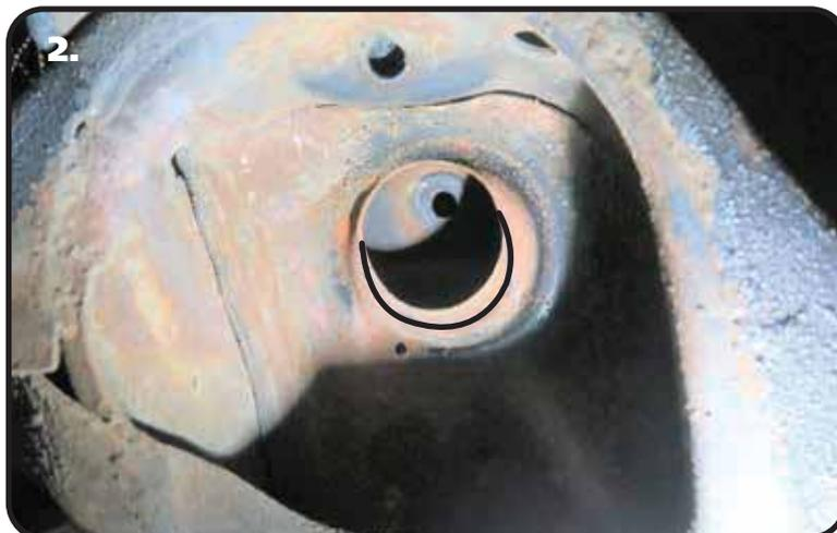
2. The CoilOver stud top will come in contact with the coil spring retainer, so it must be opened up towards the engine. **Image 2** has a white line illustrating where to cut the opening for stud top clearance. A die grinder works well here.
