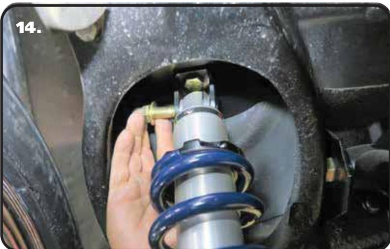
**14.** Insert the shock into the upper mount, lining up the holes of the mount and shock bearing/spacers. Install a 1/2" flat washer on a 1/2"-13 x 2 1/2" bolt. Insert the bolt/washer into the upper mount/shock. Install a 1/2" flat washer and 1/2"-13 nylok nut and Torque to 50 ftlbs.
