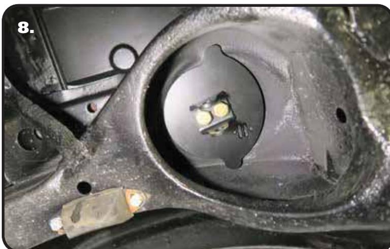
8. Install a 1/2"-13 nylok nut on each of the bolts sticking through the frame and upper clamp plate. Torque the hardware to 75 ftlbs. Repeat for the second side of the car.
