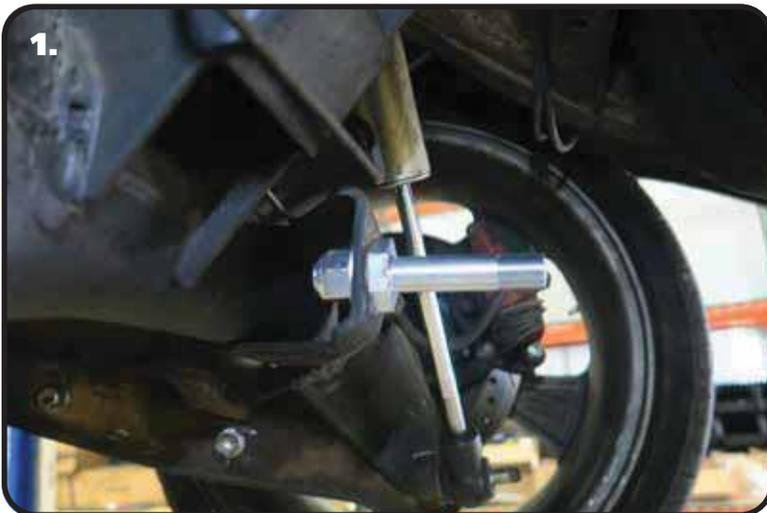
1. Bolt the new panhard bar stud into the OEM location of the axle using the 9/16" flat washer and 9/16"-18 Nylok nut supplied in the kit. Torque to 95 ftlbs.
