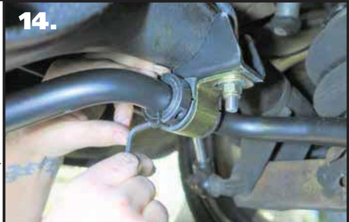
**14.** Install the locking rings on the inside of each bushing assembly. Use a hex key to take the locking ring apart. Reassemble it on the bar positioned next to the outside of the bushing assembly. Push the locking ring up against the bushing assembly and tighten.
