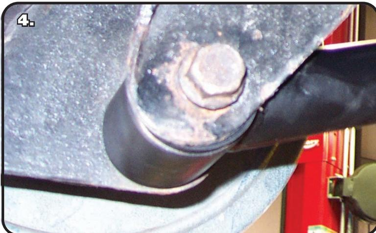
4. Attach to rear of the lower StrongArm to the frame using the 1/2" x 3 1/2" bolts and Nylok nuts supplied.
