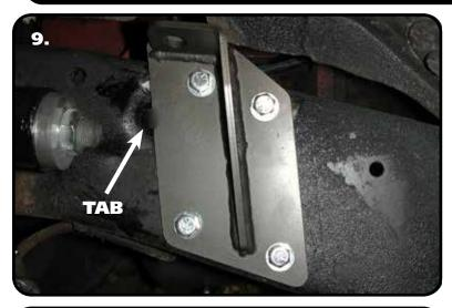
**9.** Place the new upper shock mount against the frame, the tab in the front of the bracket will slide into the factory shock stud hole. Position the bracket so that the bottom of the bracket is parallel to the bottom of the frame. Using the bracket as a template, mark an drill four 3/8" holes in the frame rail. Secure the bracket to the frame using four 3/8" x 1 ¼" bolts, Nylok nuts and flat washers. Torque the hardware to 23 ft-lbs.
