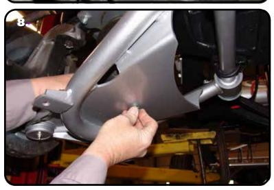
**8.** Fasten the air spring to the lower control arm using a 3/8" x 3/4" bolt, lock washer and flat washer. Torque the bolts to 23 ft-lbs.
