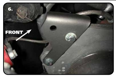
**Note:** It is acceptable to let the suspension bottom on the air spring. However, if your tire hits the inner fender well before the air spring bottoms out, this bump stop must be installed.
