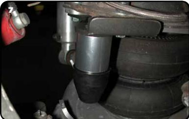
**7.** Bolt the bump stop spacer to the plate using a 3/8"-16 x 3/4" bolt, 3/8" split lock washer, & 3/8" flat washer. Torque to 12 ft-lbs. Thread the bump stop into the end of the spacer.
