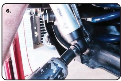
**6.** Jack the control arm up to seat the CoilSpring and attached the bottom of the shock.
