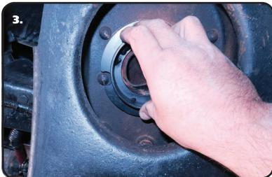
3. The Upper Coil Spring Seat is notched for a Rivet in the OEM Seat. The Notch MUST be lined up with the Rivet when installing the CoilSpring/Seat Combo.
