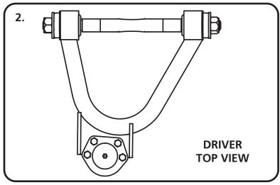
**2.** Diagram "2" shows the Driver Upper Control Arm. This is looking at the control arm from the top.
