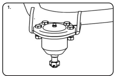
**1.** Install the balljoints into the upper control arm with the hardware supplied with the balljoint. The upper balljoint goes in from the top side of the control arm. The gussets on the balljoint plate point up. Torque the hardware to 20 ftlbs.
