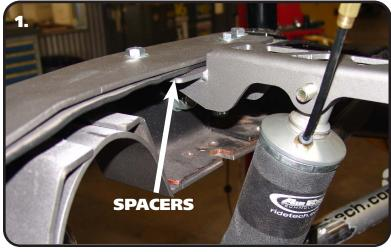
THIS KIT WILL BE INSTALLED IN CONJUNCTION WITH THE REAR TRAILING ARM KIT. WOOD BED FLOORS HANG DOWN LOWER THAN THE METAL BED FLOORS REQUIRING THE SHOCK CROSSMEMBER TO BE SPACED DOWN TO CLEAR THE FLOOR
