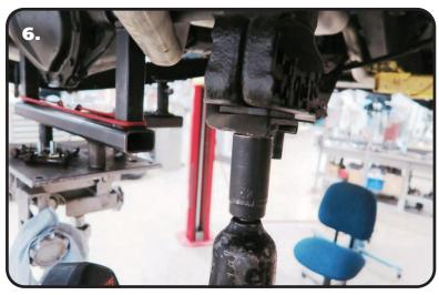
6. Remove the OEM lower shock mount by removing the u-bolt nuts. IF INSTALLING THE STREETGRIP PANHARD KIT, INSTALL THE SPACER BLOCKS AT THIS TIME. REFER TO THE PANHARD KIT INSTRUCTIONS FOR THE PROPER PROCEDURE. Retain the OEM hardware if not installing the StreetGrip Panhard Kit.
