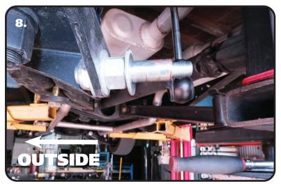
**8.** Install the supplied Shock stud in the Lower Shock Mount. The stud should be installed with the STUD pointing to the center of the truck. Install a 5/8" Washer (supplied with stud kit) on the 5/8"-18 Thread side of the Stud and insert it into the Shock Bracket. Install a 5/8" Washer and Nylok Nut on the threads and tighten. Do this for both shock brackets, installing the Studs with the small threads pointing to the center of the truck.
