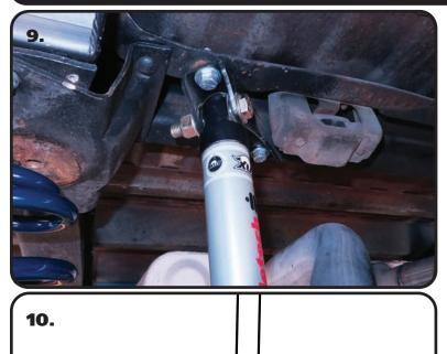
**9.** The Shock is mounted in the Upper Mount with the BODY UP. It is held in place with a  $1/2"-20 \ge 3/4"$  Hex Bolt & 1/2"-20 Nylok with a 1/2" Flat Washer on each side of the bracket.
