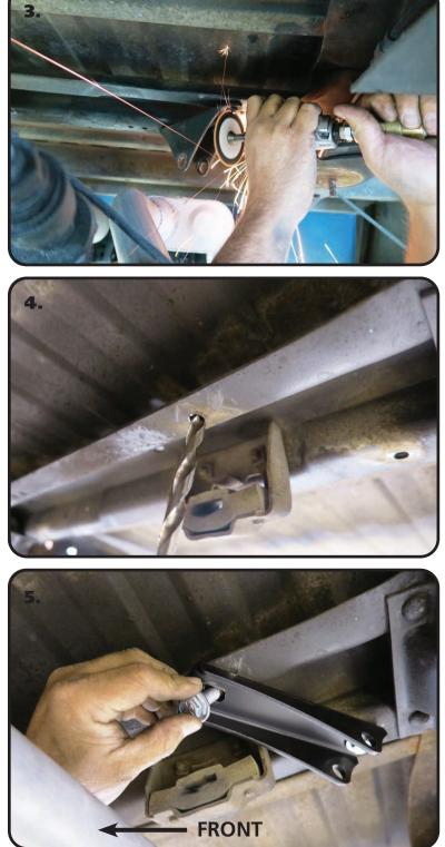
**3.** The rivets holding the OEM upper shock mount will need to be removed. One way is to cut a "+" in the head of the rivet and chisel the 4 pieces of the head off the rivet, then knock the rivet out of the frame with a hammer and punch. They can also be drilled out.
