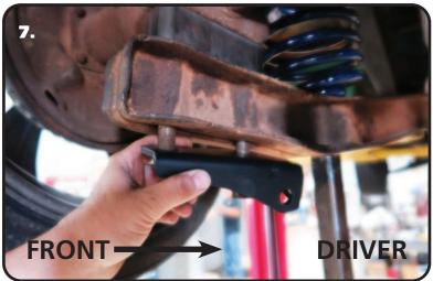
**7.** Install the Lower Shock Mount on the U-Bolts sticking through the bottom side of the trailing arm. The shock mounting hole should be positioned with the hole to the front and to the inside of the truck. Once the Mount is installed, install a 3/4" Flat Washer and 3/4"-16 Nylok Nut on each leg of the U-Bolts. Tighten the Nylok Nuts to 350ftlbs.
