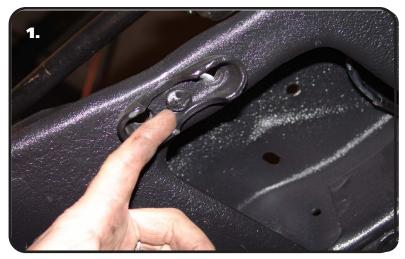
**1.** The lower control arm is installed using the factory U-bolts and nuts. The lower control arm is located by a pin that is in the center of the front u-bolt cradle. This pin will go into the hole in the control arm shaft to help locate the control arm. Torque the u-bolt nuts to 45 ft-lbs
