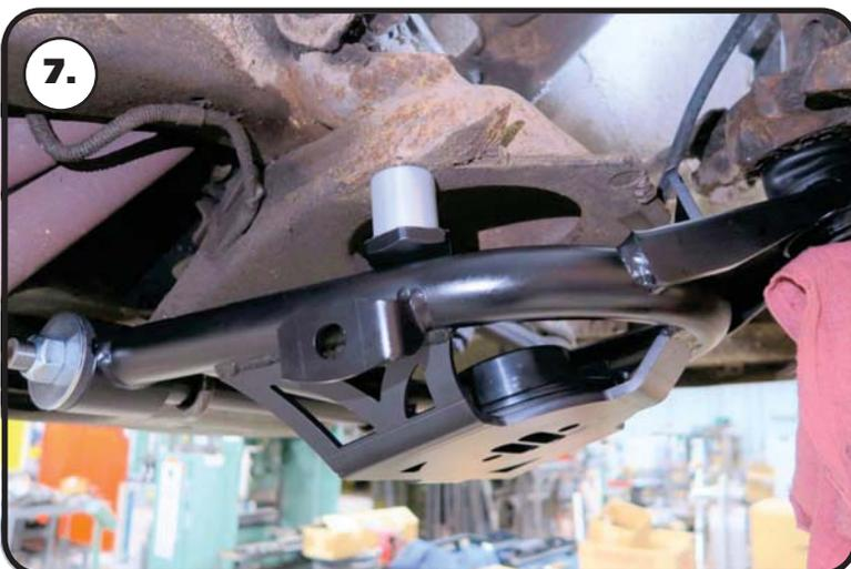
**7.** Swing the control arm up to help determine the proper location of the bump stop. The bump stop needs to contact the front tube of the control arm with the aluminum spacer sitting flat against the frame. Mark the outside edges of the spacer as you will need to drill a 3/8" hole at the center of the location.
