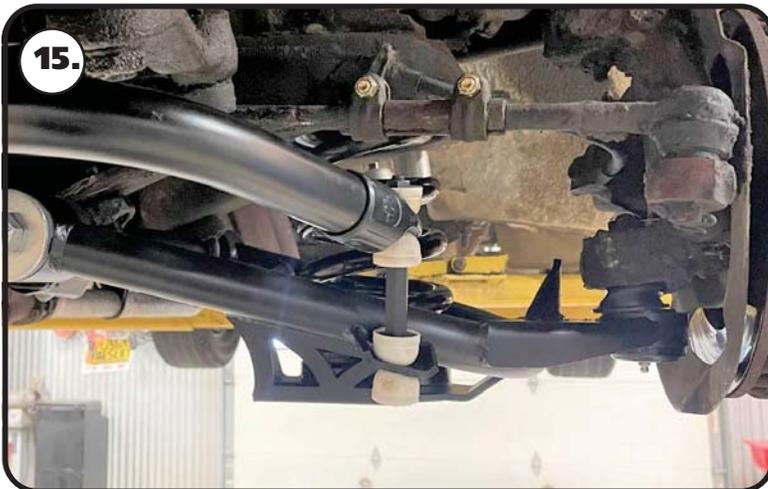
**15.** Attach the Ridetech sway bar to the lower control arm.
