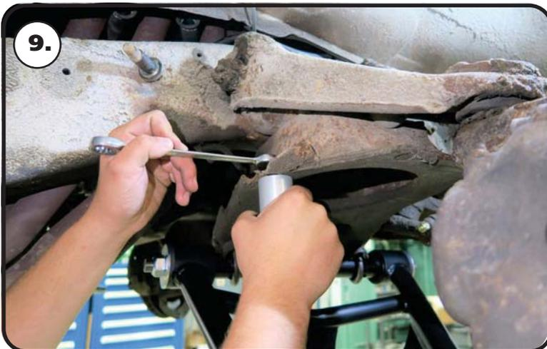
**9.** Install a 3/8" split lock washer & 3/8" flat washer on a 3/8"-16 x 3/4" bolt. Apply red loctite to the threads of the bolt. Insert the bolt in the drilled hole by reaching into the coil spring hole. Align the bump stop spacer with the bolt and thread it into the spacer. Tighten the bolt to 12 ft-lbs.
