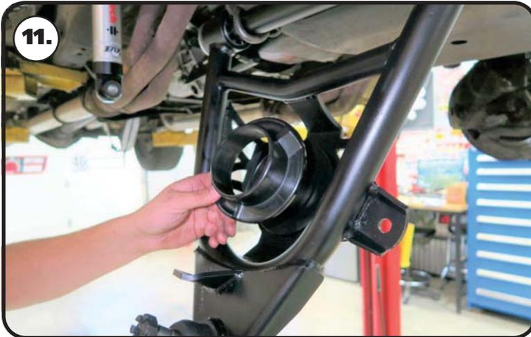
**11.** Place the coil spring isolator over the ring of the control arm.
