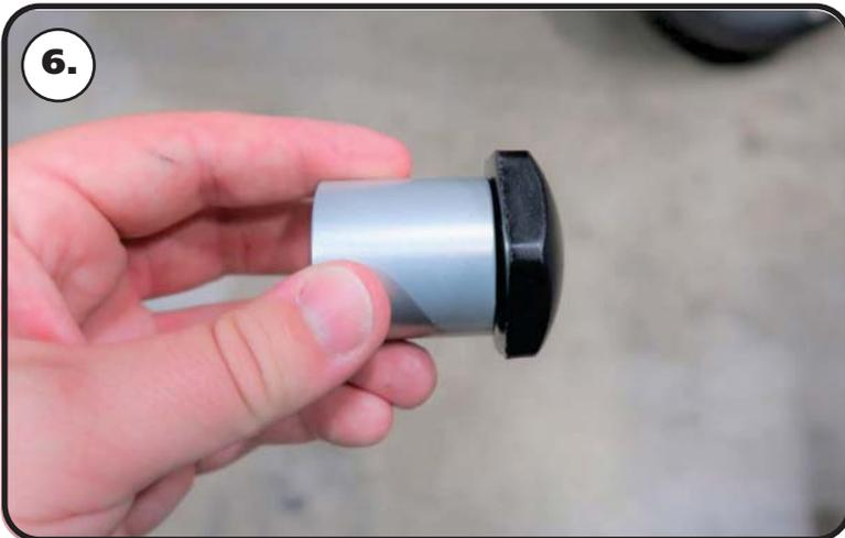
**6.** The kit includes new bump stops. **Steps 6-9** will help guide you in the installation of the bump stops. The bump stop will be installed at the rear inner edge of the coil spring opening. **Image 7** shows the bump stop installed as a reference. A hole will need to be drilled to attach the bump stop to the frame.
