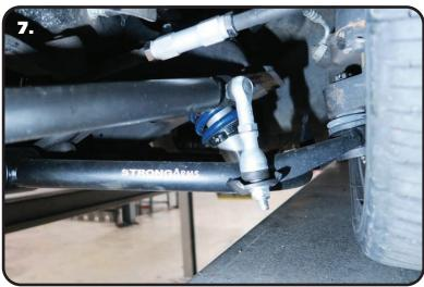
**7.** Attach the PosiLinks to the MuscleBar and StrongArm using a 7/16" SAE Flat washer on each side of the arm on the MuscleBar and each side of the bracket on the StrongArm. The 90 degree PosiLink needs to be installed with the THREADS POINTING IN TOWARD THE FRAME. Install 12mm Nylok nut on each posilink and tighten down. Torque to 50 ftlbs.
