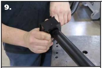
**9.** Open the sway bar bushing at the split and slide it **OVER** the swasy bar. Do this for both bushings.
