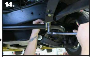
**9.** Torque the sway bar mounting hardware to 30 ftlbs.
