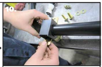
**10.** Next, slip the bushing straps over the sway bar bushings.
