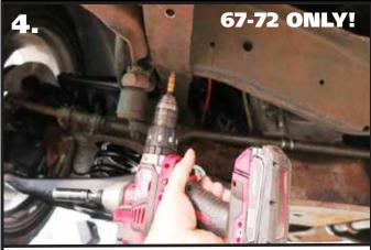
**4.** Remove the rivet from the bottom of the frame rail. This can be done by cutting the rivet head off and driving it out or by drilling it out. This cross member is located in front of the suspension cross member.
