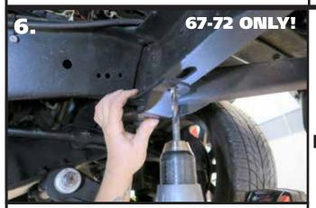
**6.** With the rear hardware installed, line up the bracket parallel with the frame rail. Use the front hole as a guide to drill a 3/8" hole in the frame.
