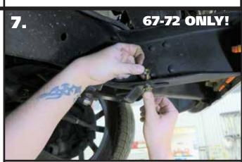
**7.** Attach the front of the bracket using a 3/8"-16 x 1 1/4" bolt, 3/8"-16 Nylok nut and a 3/8" Flat Washer on top and bottom. Repeat on the other side and tighten hardware. **SKIP TO STEP 9.**
