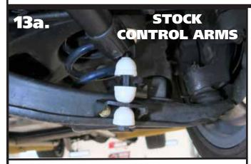
**13a. STOCK CONTROL ARMS** Install the SHORT end links using **Diagram 1** as a reference. Install both end links before tightening the end link hardware. Tighten the end link barrel nut until it is flush with the end of the bolt, and then tighten it 2-3 more complete rounds.
