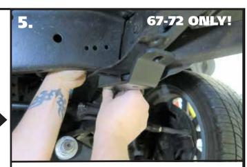
**5.** Attach the rear hole of the frame mounting bracket to the frame using the rivet hole. The end of the frame bracket with the angled bends goes forward. Attach the bracket using a  $3/8"-16 \times 1 /4"$  bolt,  $3/8"-16 \times 1 /$
