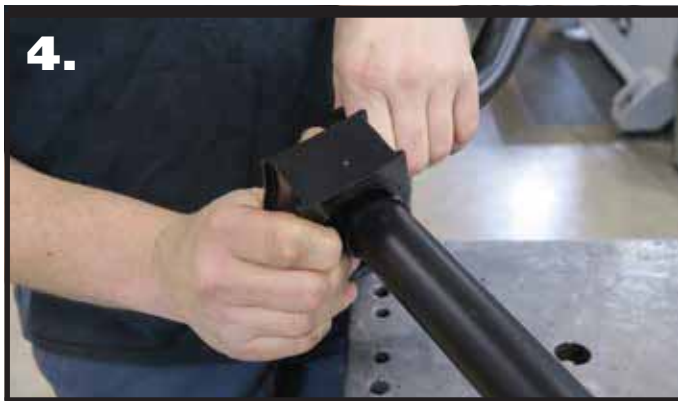
4. Open the sway bar bushing at the split and slide it OVER the swasy bar. Do this for both bushings.
