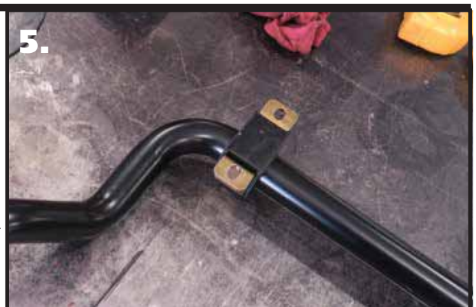
5. Slip the Bushing Straps over the Sway Bar Bushings.
