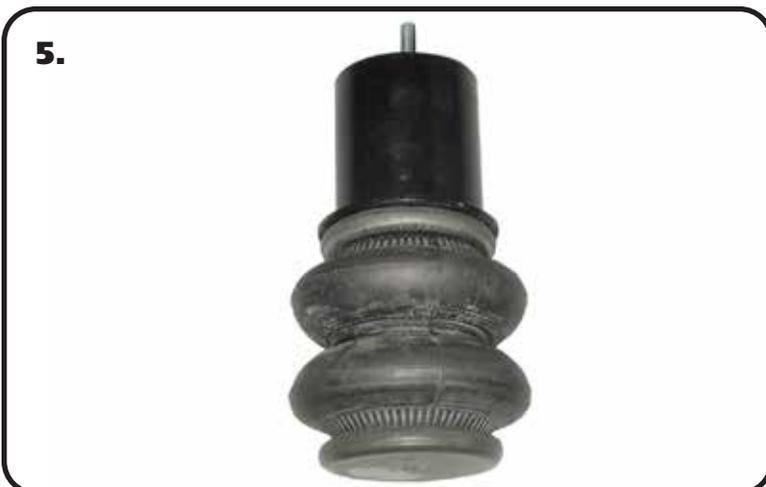
5. Apply thread sealant to the air fitting and screw it into the air spring. Assemble the upper cup bracket to the air spring, using 3/8"-16 Nylok nuts and 3/8" flat washers. Torque the 3/8" nuts 15-20 ftlbs. Thread the 8" stud into nut welded to the bottom of the cup bracket.
