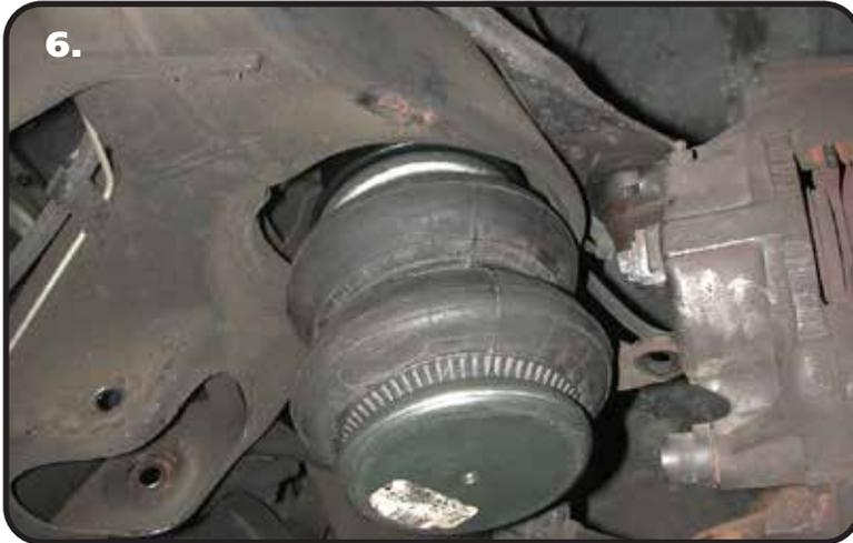
**6.** Place the assembly up into the upper coil spring pocket; the stud will go through the factory shock hole. Fasten with a 7/16"-14 Nylok nut and 7/16" flat washer. Tighten the nut enough to hold the airspring/cup solidly in place.
