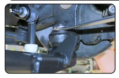
**5.** Attach the Spindle to the control arms.
