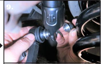
**9.** Insert the 90 degree end link/t-bushing into the swaybar end with the threads pointing toward the coilspring. Install a 2nd t-bushing with the small diameter into the swaybar. Install the nut and torque. Do this for both sides.
