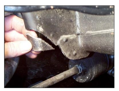
1. The upper coil spring bucket must be trimmed for air spring clearance. The trimmed piece will measure approx. 1 3/4 x 1 3/4. A die grinder and a cutoff wheel will do the job nicely. The objective here is to create clearance for the air spring. Check this area VERY carefully for abrasion against air spring.
