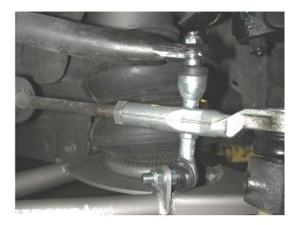
2. Install the lower air spring mounting plate into the lower control arm using the oem sway bar attachment hole as the primary locater. The remaining attachment holes will then be drilled so the plate can be securely fastened to the control arm.
