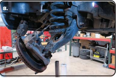
**8.** Support the lower control arm with a jack and disconnect the upper ball joint from the spindle, SLOWLY lower the control arm to relieve tension from the coil spring. Remove the coil spring from the truck.
