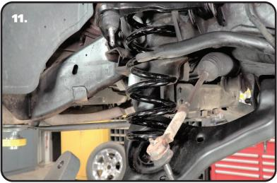
**11.** Insert the coil spring/seat combo into the OEM coil spring pocket. Twist the spring on the upper seat to get the bottom of the coil spring lined up with the receiver in the control arm. The end of the coil spring needs to be nested into the receiver area of the control arm. Slowly jack the control arm up.
