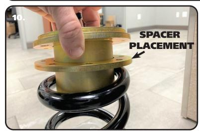
**10.** The coil spring seat is positioned on the top of the coil spring with the center ring inserted into the coil spring. Use the guide on Page 2 for determining if you should install spacer(s).
