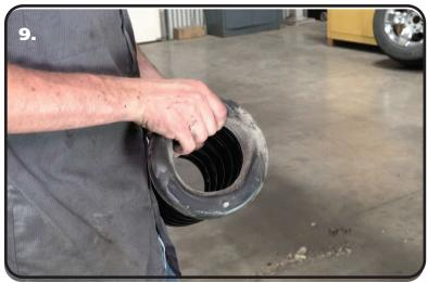
**9.** Remove the spring rubber from the OEM spring and install it on the new coil spring.
