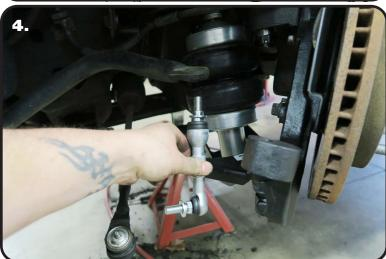
**4.** Install the T-Bushing on the Straight PosiLink end with the Large OD against the PosiLink. Insert the assembly into the swaybar with the threads pointing up. Install a 7/16" Flat Washer followed by a M12-1.75 Nylok Nut. Torque to 50 ftlbs.
