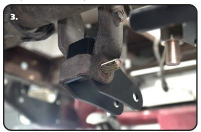
**3.** This kit includes new lower shock mounts to correct the angle of the shocks. They attach to the OEM shock mounts. Slip the lower mount into the OEM shock mount lining up the 2 side holes with the OEM shock hole. You will need to drill the rear hole into the OEM mount. Use the bracket as a template to mark the location of the hole that will need to be drilled.
