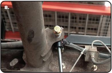
**8.** Insert the shock into the OEM upper mount. Install a 9/16" flat washer on a 9/16"-18 x 3" bolt, insert the bolt/washer through the upper mount. Install a 9/16" Washer and 9/16"-18 Nylok Nut on the threads sticking through the mounts/spacer. Tighten the 9/16" hardware to 100 ftlbs. Repeat for the other shock bracket.
