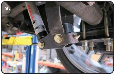
**9.** Install a 1/2" flat Washer on a 1/2"-13 x 2 3/4" Bolt. Line the center of the inner sleeve of the shock with the mounting holes in the lower shock bracket. Insert the bolt/washer through the lined up holes. Install a 1/2" Flat Washer and 1/2"-13 Nylok Nut on the threads sticking through. Torque to 50 ftlbs.
