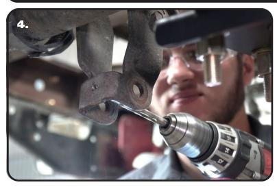
**4.** You will need to remove the new mount to be able to drill the hole in the OEM mount. Use a 5/16" drill bit to dill the hole.
