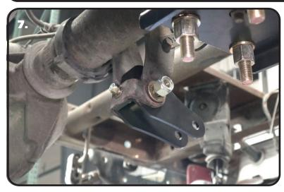
**7.** Install a 9/16" flat washer on a 9/16"-18 x 3 1/4" Bolt, insert the bolt/washer through the lower mount, OEM mount, and spacer. Install a 9/16" Washer and 9/16"-18 Nylok Nut on the threads sticking through the mounts/spacer. Tighten the 5/16" hardware to 25 ftlbs. Tighten the 9/16" hardware to 100 ftlbs. Repeat for the other shock bracket.
