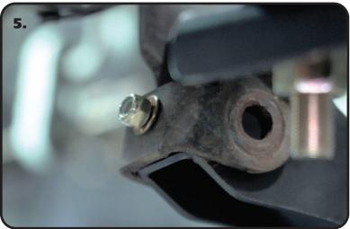
**5.** Reinstall the new shock mount, aligning the holes. Install a 5/16" Flat Washer on a 5/16"-18 x 1" Bolt and insert in through the small hole with the bolt head on the INSIDE of the new shock mount. Install a 5/16" flat washer followed by a 5/16"-18 Nylok Nut on the threads of the bolt sticking through the bracket. Do not tighten at this time.
