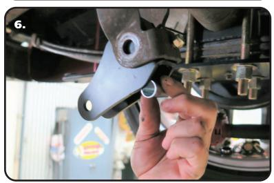
**6.** Insert the spacer (1.312" Long) into the new shock mount. Align the center hole with the OEM shock holes.
