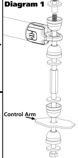
Tighten the end link barrel nut until it is flush with the end of the bolt, and then tighten it 2-3 more complete rounds.
