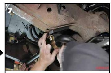
**7.** Slide the SwayBar into position on the S10 with the SwayBar arms above the tie rods. Install a 3/8" Lock Washer & 3/8" Flat Washer on the 3/8"x 3/4" Hex Bolts. Do **NOT** Complete tighten the Hardware, it will be left partially loose until the End Links are installed.
