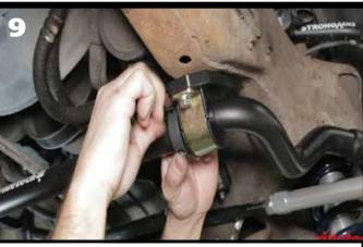
**9.** Torque the SwayBar mounting hardware to 30 ftlbs. Install the locking rings on the inside of each bushing assembly. Use a hex key to take the locking ring apart. Reassemble it on the bar positioned next to the inside of the bushing assembly. Push the locking ring up against the bushing assembly and tighten.
