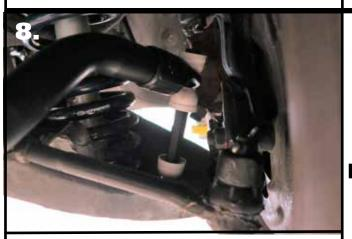
**8.** Install the End Links using **Diagram 1** as a reference. Install both end links before tightening the end link hardware. Tighten the end link barrel nut until it is flush with the end of the bolt, and then tighten it 2-3 more complete rounds.
