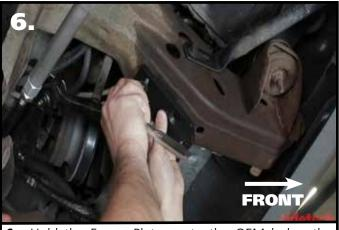
**6.** Hold the Frame Plate up to the OEM holes, the Counter Sunk holes will line up with the OEM threaded holes. The Plates are positioned with the threaded holes offset to the **FRONT and INSIDE of the truck**. Apply Red Loctite to the Flat Head Bolts. Torque Hardware.
