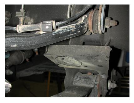
4. To reach maximum drop the bump stop and bump stop cup must be removed. This can be done with a cut off wheel. This picture shows the bump stop bracket after removing the cup.
