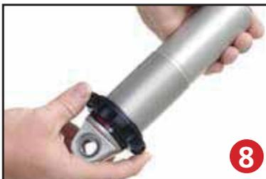
First, using the supplied lower adjuster nut (803-00-199) thread the nut onto the shock from the bottom side as seen in figure 8. Remove the plastic pellet that is in the split of the adjuster nut.
