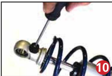
Before the upper spring mount can be installed screw the adjuster knob on the upper eye mount to the firmest setting (clockwise) as seen in figure 10. Then remove the Knob by holding it while removing the center screw.
