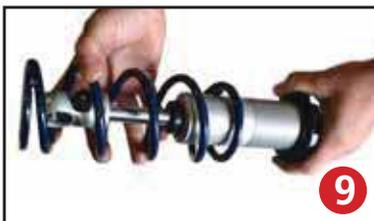
Next, install a delrin washer then coil spring over the top of the shock as seen in figure 9.
