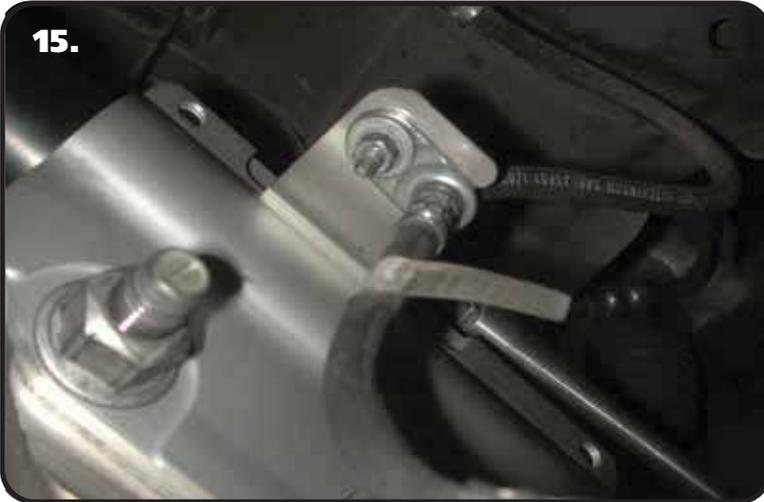
15. Using the factory hardware, attach the brake line to the mount on the strut.
