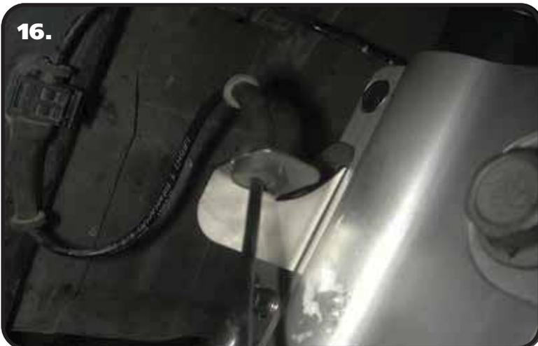
16. Slide the ABS wire into its mount on the strut.
