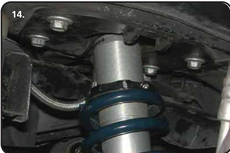
**14.** Install the Coilover/Upper Mount assemble into the car using the factory hardware. There is a Driver and Passenger upper bracket. These brackets are marked accordingly. Once the assembly is installed in the car, rotate the shock eyelet so that the adjuster knob is towards the outside of the car.
