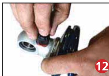
Install upper spring mount retainer clip (803-00-199) into the groove on the upper eyelet as seen in figure 12. Then, reinstall adjuster to complete assembly.
