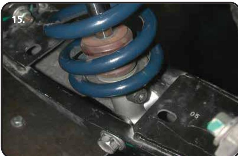
**15.** Install the (90002381) spacers(1) into the bearing in the shock eyelet(2). Align the shock eyelet with the factory mounting hole. Reinstall the factory hardware and torque to 50 ftlbs to eliminate any gaps between the spacers and control arm.
