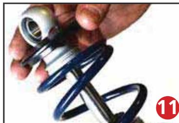
Once the knob is removed slide a Delrin washer over the eyelet. Next, slide the upper spring mount (803-00-199) over eyelet as seen in figure 11.
