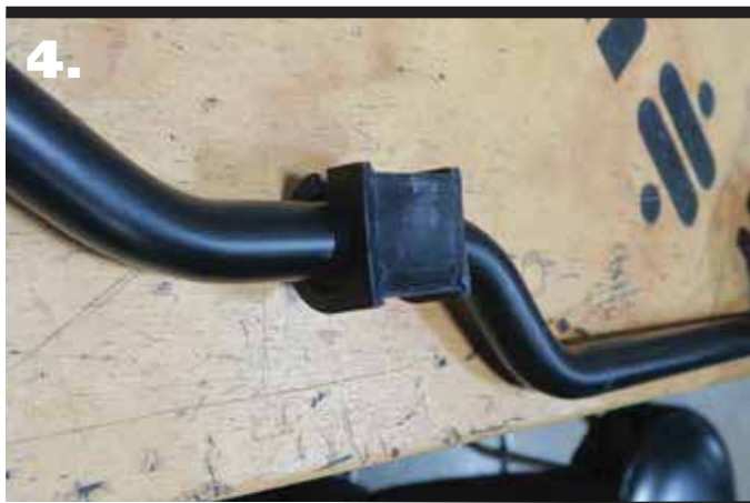
4. Open the Sway Bar Bushing at the split and slide it on the sway bar.. Position it in the area that the bushing will ride based on the location of the stock swaybar. Do this on both ends of the swaybar.
