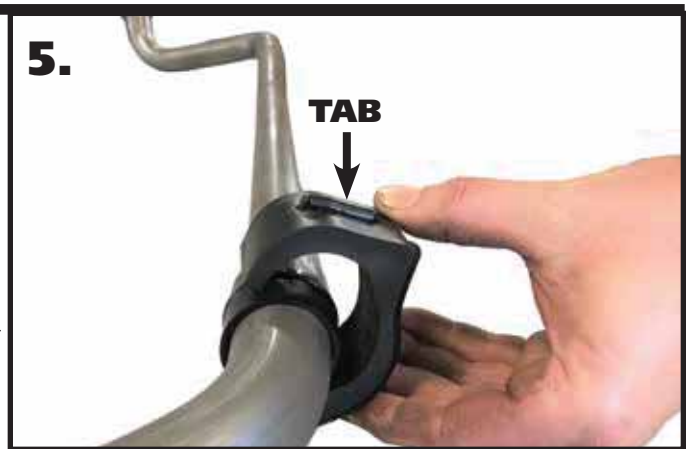
5. Open the Sway Bar Bushing at the split and slide it OVER the Delrin Liner. The Bushing needs to be installed with the TAB upward and the radius to the rear. Do this on both Delrin Liners. Images 5 & 6 illustrate the correct positioning of the bushings.
