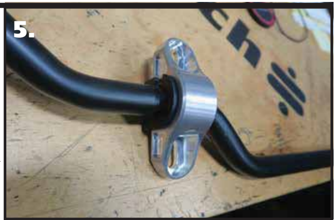
5. Slip the Bushing Straps over the SwayBar Bushings.
