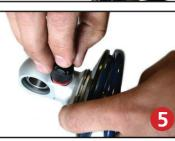
Install upper spring mount retainer clip (803-00-199) into the groove on the upper eyelet as seen in figure 5. Then, reinstall adjuster to complete assembly.
