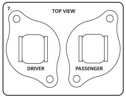
7. New Upper Mounts are included to replace the OEM mounts. The Upper Mount will be replaced with mounts included in the Shock Kit. When these mounts are installed correctly, the Upper Mounting Bolt will be PARALLEL with the Lower Mounting Bolt.
