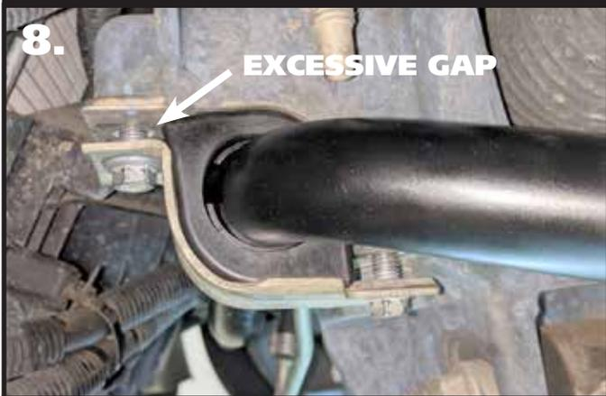
**8.** If you are experiencing an excessive gap between the cradle and bushing straps, install the (4) supplied spacers between the strap and cradle. Excessive gap would be 5/16" or more.
