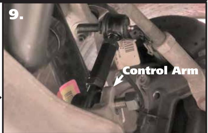
**9.** Thread the jam nuts all the way up the threads of the 90 degree ends. Evenly thread an end link into each end of the spacer until they bottom out. Adjust the endlinks out until they are pointing in opposite directions of each other. Attach the Linkage to the OEM sway bar tab on the lower control arm with the threads pointing forward. Torque the hardware.
