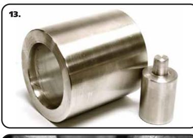
**13.** With the upper reattached, it is time to do the Lower Control Arm. Ridetech sells tool 85000006 to aid in removal of the bushings. The Tool is 2-sided with a large opening for the Lower Bushings and the opposite side being smaller for the Rear Upper Bushings. It comes with a Mandrel to insert into the center sleeve for pushing the Bushings out of the Control Arm.
