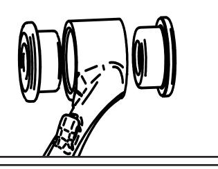
**10.** Press a set of bushings into each opening of the upper control arm. A bench vise can be used to do this.
