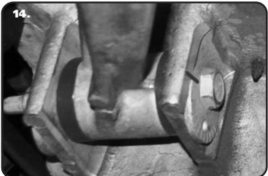
14. Before removing the Lower Control Arms, use a Marker or something similar to mark the Lower Control Arm Eccentrics. Also, mark the location of the bolts. The marks will get the Alignment close, but Ridetech recommends getting the alignment checked after the install is completed.
