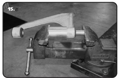
**15.** Remove the Lower Control Arm. Using the Ridetech tool (with large side over bushing) and a Bench Vise, push out the original Bushings. Clean out the opening of any debris that may have been left behind.
