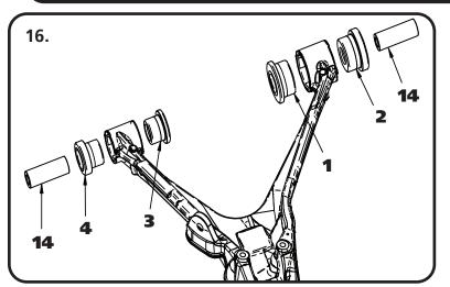
**16.** Using the Diagrams on Page 2 & 3, Insert the correct Bushings in the correct locations using a Bench Vise to push them in. Push the Bushings in followed by the correct Inner Sleeve. The Front Lower uses Bushing 1, 2, 3, 4, and Inner Sleeve 14
