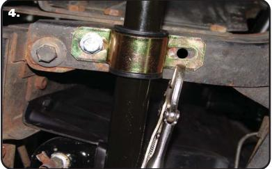
**3.** Insert the MuscleBar into position by sliding it between the bumper support and the frame rail. With the MuscleBar slid in place, install the mount bushing onto each end of the MuscleBar followed by the mounting strap.
