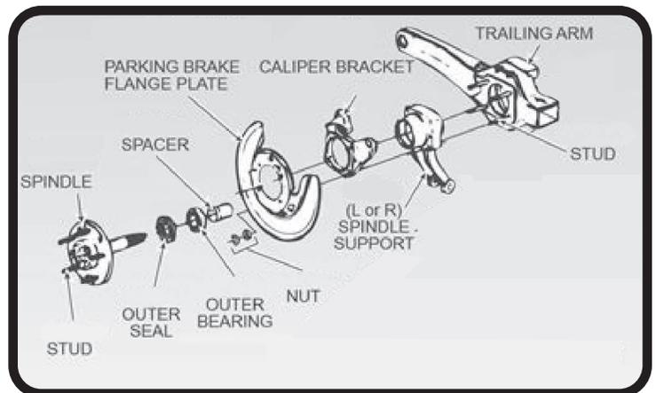
The caliper brackets are installed on the studs of the trailing arm, on top of the spindle support. The above pictures show the driver side.
