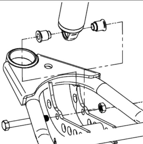
3. Install a spacer on each side of the lower Coilover. Slide the shock with the spacers installed into the lower control arm. Raise the arm up to line up the holes in the bushing with the 1/2" hole in the control arm straps and hold it in place while you install the 1/2" x 3 1/4" bolt and 1/2" Nylok nut. Tighten the upper and lower shock bolts.
