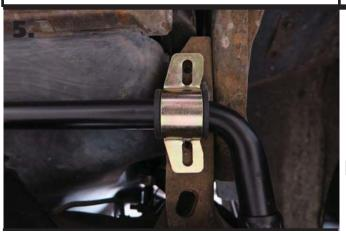
**5.** Slide the Sway Bar into position on the car. The sway bar is installed in the OEM location. You may need to move the bushing/straps on the sway bar to line them up with the OEM mounting holes.
