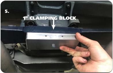
**5. 63-78 CORVETTE WITH 2 1/4" LEAF SPRING!** The kit contains a 1" thick clamping block that needs to be positioned between the composite leaf spring and OEM clamping plate. The clamping block has a center hole that the leaf spring pin will nest into. The pin of the clamping block will be pointing down.
