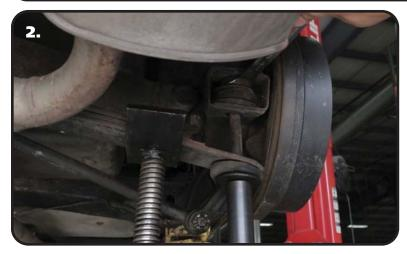
**2.** Use the jack to raise one end of the leaf spring enough to take tension off the leaf spring linkage bolt. Remove the linkage. Slowly release the jack. Repeat on the other side.
