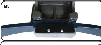
If you are looking for a level car, start with the block on the bottom side of the leaf spring. If you like the rear of the car higher, put the block on the top side of the leaf spring. The leaf spring bolt spacers are 1/2" tall and will change the ride height approximately 3/8" per set of spacers.
