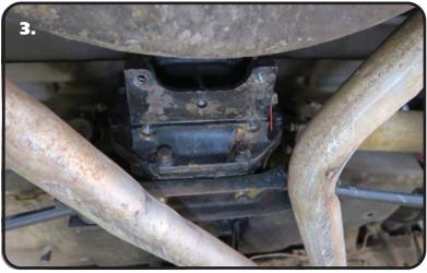
**3.** With both ends of the leaf spring disconnected from the trailing arms, remove the center clamping plate. Retain the clamping plate for installation of the new leaf spring. On 80-82 Corvettes, you will need to remove the shield that is below the leaf spring clamp.
