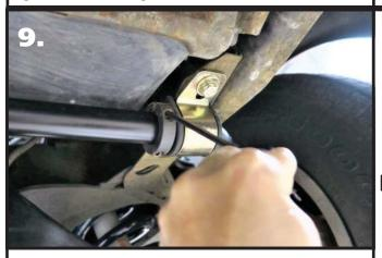
**9.** Install the Locking Rings on the sway bar. They will be positioned against the inside of the sway bar bushings. You will need to disassemble the locking rings to install them on the sway bar. Tighten the hardware with a hex wrench.
