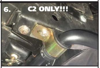
**6. C2 ONLY!!!** The C2 Corvette requires a Spacer to be used between each Sway Bar Bushing and the frame. Be sure to get the offset the same direction as the bushing strap. The holes should be offset toward the bend of the sway bar.
