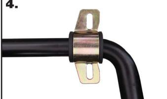
**4.** The Bushing Straps have the mounting holes that are offset. **The Mounting Holes need to be closest to the bend of the sway bar.** Slip the Bushing Straps over the Sway Bar Bushings.
