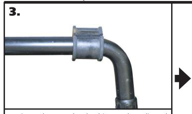
**3.** Open the sway bar bushing at the split and slip it **OVER** the sway bar. Do this for both bushings
