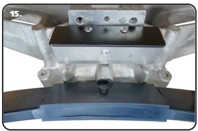
**15. 80-82 CORVETTE!** Hold the clamping block in place and put the leaf spring in place. THE CENTER LOCATING PIN NEEDS TO BE INDEXED INTO THE HOLE OF THE CLAMPING BLOCK.
