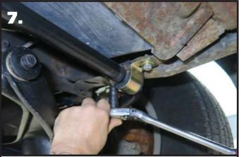
7. Again, the mounting holes need to be closest to the bend off the sway bar.. Install a 5/16" Lock Washer & 5/16" Flat Washer on (2) 5/16"x 1" Hex Bolts. Insert the hardware through the OEM swaybar mounting holes, threading the hardware in to the mount. Do NOT tighten the mounting hardware at this time.
